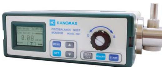
In contrast, a piezobalance dust monitor operates by electrically charging the particulates it takes in. The charged particulates are then deposited on a piezocrystal. By measuring the change in frequency of the crystal the monitor is able to determine the mass concentration of the particulates. Since the actual mass concentration is measured there is no need for a K-factor with this type of monitor.
