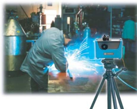
It is possible to estimate the K-factor if the mass concentration of the particulates being monitored is known, but as each environment is unique this method will not provide the greatest possible accuracy. For precise measurements it's always best to sample the particulates at the actual measuring site at the exact location the dust monitor will be placed when monitoring.
