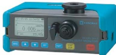
Light Scattering Monitors are the most common in the industry. Dust is introduced to the monitor via a particle inlet which funnels the particulates toward a laser beam. The particles pass through the beam in single file and the instrument measures the concentration via the amount of light that is scattered as the particle passes through the beam.
